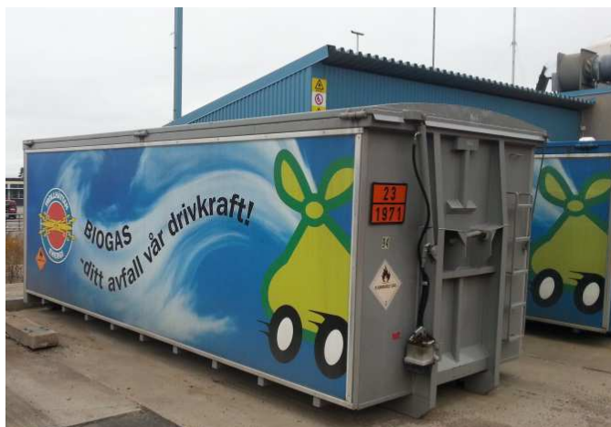
Figure 3-1. Container used for transportation of compressed vehicle gas in Sweden. The container is filled with high pressure gas cylinders
